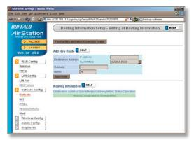
To configure a route manually, enter its Destination Address and Gateway. Enter a maximum number of hops allowable in Metric and click Add.
