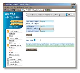
You may disable Network Address Translation and IPsec passthrough by unchecking the appropriate *Enable* boxes. If you have a DMZ, enter its IP address in the *IP Address of DMZ* box. Incoming packets containing no recognizable destination port information will be redirected to the DMZ's IP address.
