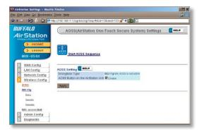
Clicking *Start AOSS Sequence* has the same function as pushing the AOSS button on the router: it initiates the AOSS process.
