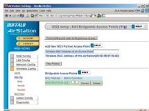
Now, you need to configure the second AirStation with the MAC address of the first one. In your browser's address field, enter "192.168.11.100". This will take you into the Web-Based Configuration Utility for the second AirStation.
