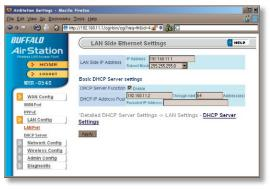
Default for the *LAN side IP address* is 192.168.11.1. To add the AirStation to an existing LAN, specify a unique IPaddress, not used elsewhere in the network.
