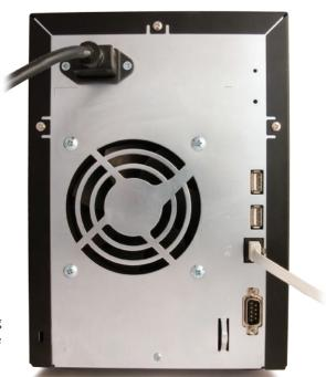
Begin setting up your TeraStation by plugging your *power cable* and *Ethernet cable* into the back of the TeraStation as shown.
