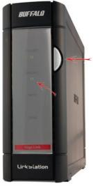
Press the *power button* on the front panel. LEDs will blink as your LinkStation boots up.
